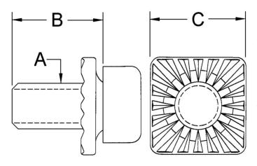
Various head types are available for all combinations shown. The Clamp-Fast is available in thread forming, self-tapping and self-centering. Sizes other than those shown below are available on special order.
